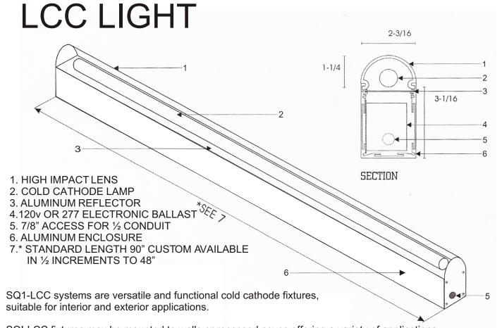
SQ!-LCC fixtures may be mounted to walls or recessed coves offering a variety of applications.
